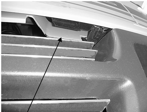
Squeeze latch handles toward hood panel and lower hood down into open position.
