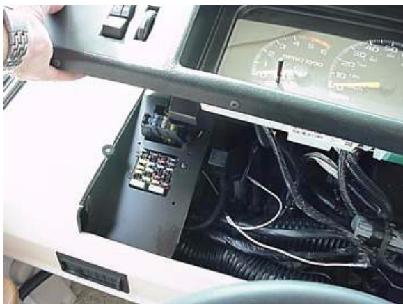
Automotive 12-Volt Fuse Panel Beneath Lift-Up Dash Pod
