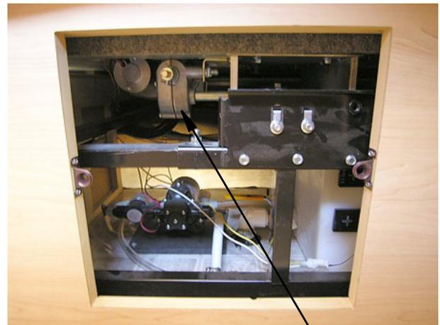
Rear Slideout Motor/Gear Location
