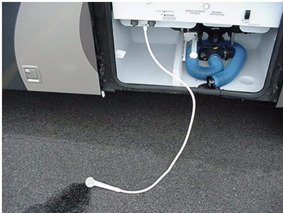
4. Turn on water pump and open all sink faucets and shower head knobs. Leave open after water stops flowing.
