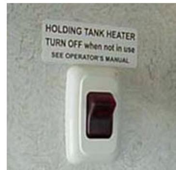
**DO NOT** operate the holding tank heaters unless you are providing a supplemental 12-volt power source to recharge the house batteries.
