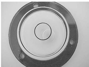
Normal vehicle leveling to provide comfort for the occupants is satisfactory for refrigerator operation.
