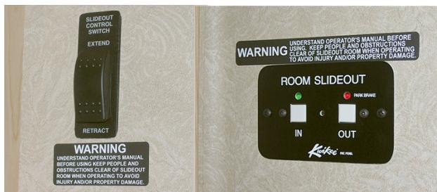
Slideout Switches (typical)
