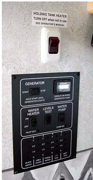
The Systems Monitor Panel provides a convenient central location for checking the condition of all utility systems in your coach. At the touch of a button this panel can display the fresh water or holding tank levels, LP gas tank level, plus the coach battery condition. You can start the auxiliary generator or turn on the water pump and water heater. Indicator lights tell you if the water pump is on or if the water heater pilot light is out.
