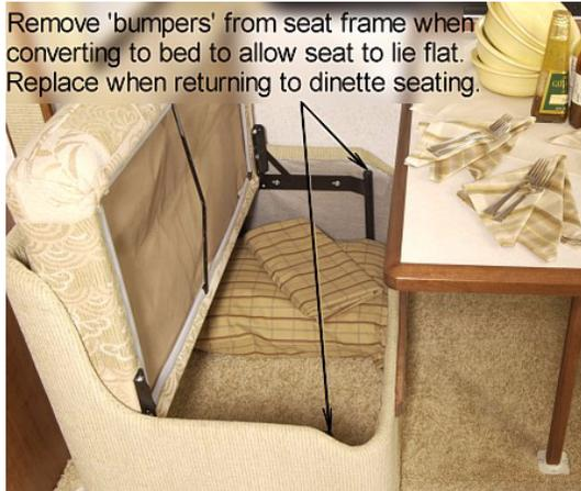
Remove 'bumpers' from seat frame when converting to bed to allow seat to lie flat. Replace when returning to dinette seating.
