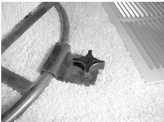
The clamp knob can be unscrewed and removed to allow you to position the chair as you desire in the living area of the coach.
