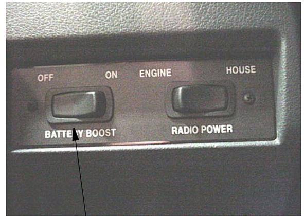
If the engine battery is dead, press and hold Battery Boost Switch ON while turning the ignition key for emergency starting power.
