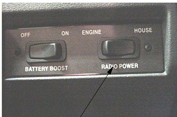
Press HOUSE to listen to the radio while parked without the ignition key on. Press ENGINE to listen while driving.
