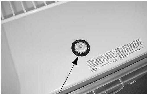
Place bubble level in bottom of refrigerator
