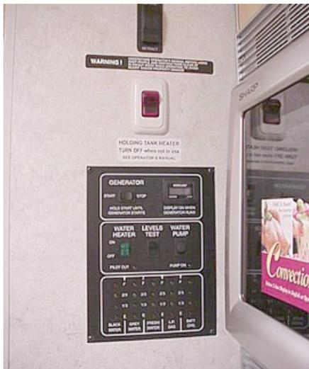
The Systems Monitor Panel provides a convenient central location for checking the condition of all utility systems in your coach. At the touch of a button this panel can display the fresh water and holding tank levels, LP gas tank level, plus the coach battery condition. You can start the auxiliary generator or turn on the water pump or water heater. Indicator lights tell you if the water pump is on or if the water heater pilot light is out.
