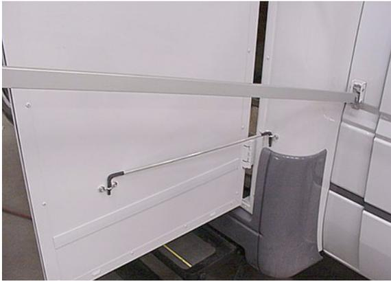
The door prop rod is stored beneath the couch (model 523H) or in the right rear exterior compartment (model 523J).
