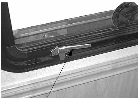
Lift latch handles upward to open.
