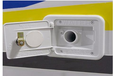
Water Tank Gravity Fill
