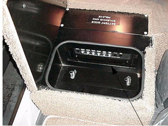
Chassis/House 12V Circuit Breakers behind cover panel in floor compartment between front seats.
