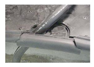
Route the cord through the notch and flip the hatch back up into place and close the compartment door.
