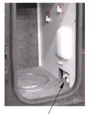
Water Line Drain Valve
