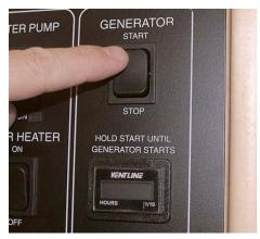
Generator Switch and Hourmeter on monitor panel
