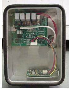
Hydraulic System Control Box on pump underside of coach near front tire
