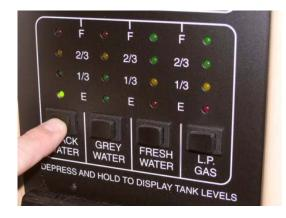
The approximate fluid levels are measured by sets of electronic sensors (detector cells) on the sides of the tanks. There is generally more fluid in a tank than indicated on the monitor panel.
