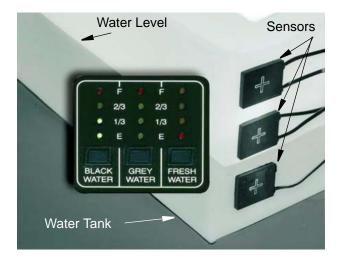
For example, if the fluid level is 1-2" below the FULL sensor, the monitor will show the level to be only 2/3 even though the tank is nearly full.
