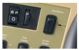
When this switch is ON, the transmission will automatically shift to the overdrive gear whenever possible for greatest fuel economy.
