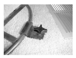
You can unscrew the knob and remove the clamp to position the chair where you desire in the living area of the coach.
