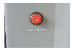
NOTE:If one of the leveling jacks should fail to retract, it can be normally retracted by opening a T-handle valve on the reservoir side of the hydraulic pump. The jacks are spring loaded to retract when hydraulic line pressure is relieved. See the Leveling System Operator's Manual included in your InfoCase for specific instructions on which valve to open and what precautions to follow. The hydraulic pump is located under the entrance step. Valves will be in same relative positions.
