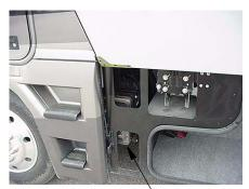
Hydraulic Pump Access \(^1\) open storage compartment door behind driver's side front tire.
