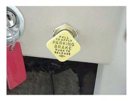
Note: Never drive your vehicle with the parking brake set. It will reduce parking brake effectiveness and cause excessive wear.
