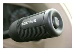
Press the button at the end of the shift lever to engage Tow/Haul Mode when pulling a trailer or tow vehicle.
