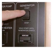
Generator Switch and Hourmeter
