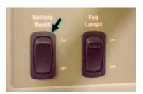
Battery Boost Switch If engine battery is discharged, press and hold while turning ignition key for emergency starting power.
