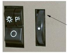
Roll panel light dimmer wheel upward fully to turn driver side map light on.
