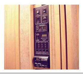
At the touch of a button this panel can display the fresh water and holding tank levels, propane gas tank level, plus the battery and house battery condition. You can start the electric generator or turn on the water pump and water heater. Indicator lights tell you if the water pump is on or if the water heater pilot light is out.
