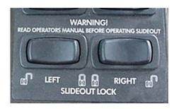
Note: Be sure locks are fully released. The room will not extend or retract if the locks are protruding more than 1/4", and you will hear the slideout hydraulic pump running in idle/bypass mode when attempting to extend or retract room.
