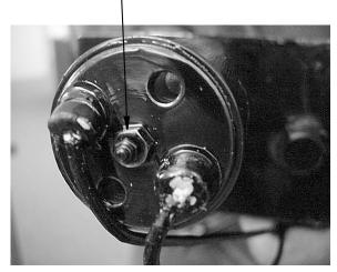
Slideout Room Solenoid Valve
