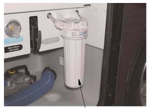
Central Water Filter System in Water Center (typical)
