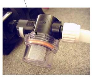
Water Pump Strainer in Water Service Center (typical)
