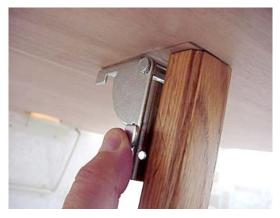
3. Remove the table from the wall support bracket by lifting the end of the table. Then lower the table to rest on the cleats attached to each dinette bench.
