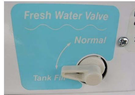
Fresh Water Valve in Tank Fill position
