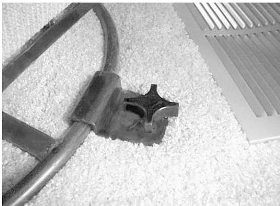
The clamp knob can be unscrewed to allow you to position the chair away from the wall.
