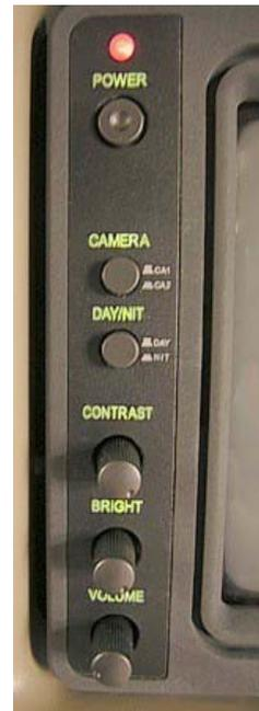
**Power** - Turn ON to activate monitor for rear viewing while driving or parked. Key must be on.
