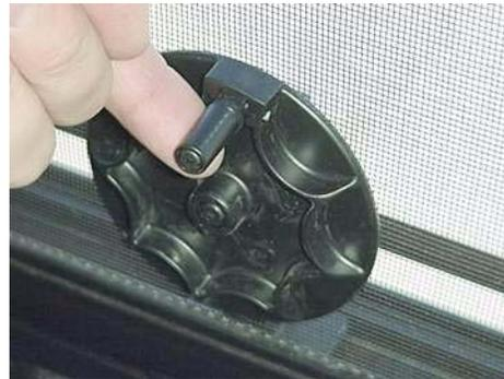
If the window will not open after three or more full turns of the knob, the glass may be stuck to the sealing gasket. Go to the outside of the coach and gently free the glass with your fingers. A periodic light dusting of talcum powder on the gasket should prevent this from recurring.
