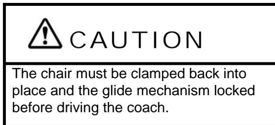
The chair has a glide-lock mechanism to prevent chair movement while the coach is moving. The glide lock is located behind the seat skirt on the rear side of the seat base mechanism.
