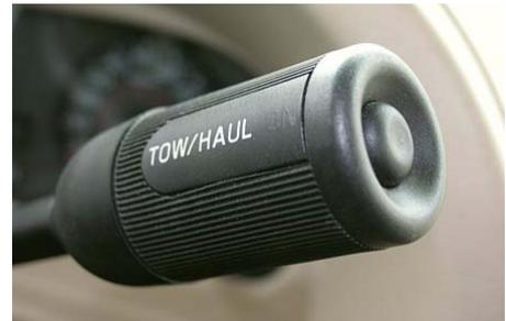
Press the button at the end of the shift lever to engage Tow/Haul Mode when pulling a trailer or tow vehicle.
