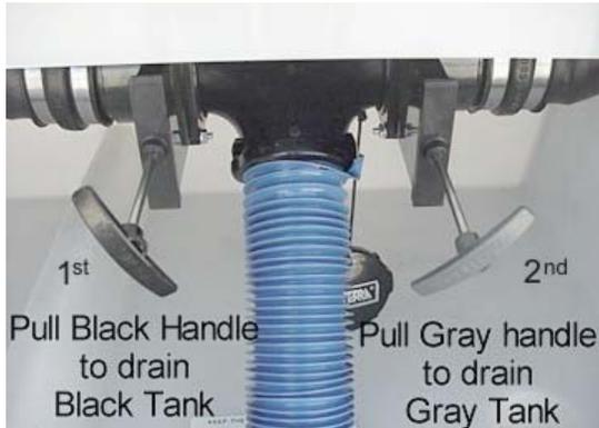
Holding Tank Dump Valves (Typical)
