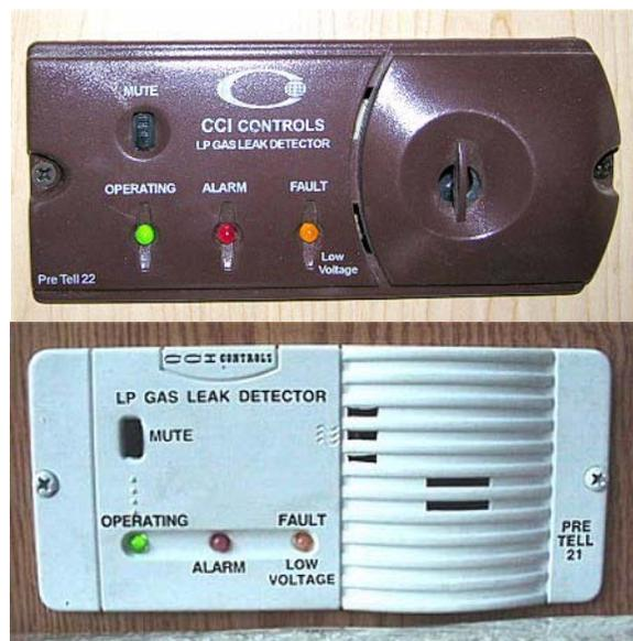
Propane Gas Leak Detectors (Typical)
