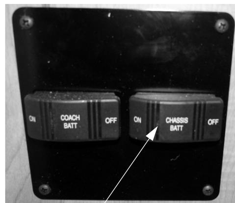
Chassis Battery Disconnect Switch
