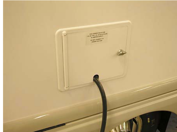
Route power cord through notch and close door while shoreline is connected to outlet.
