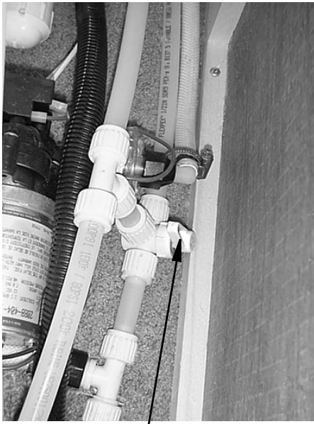
Waterline Drain Valve (Typical)
