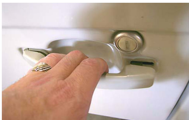
Pull door handles out to unlatch door
