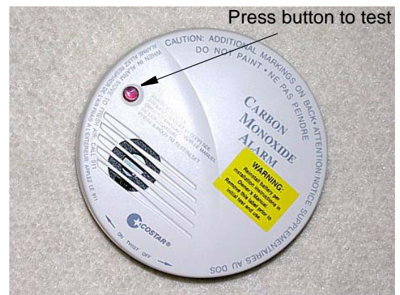
Carbon Monoxide Alarm
