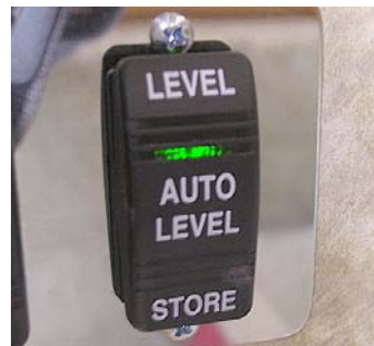
Auto Level Switch inside Entrance Door (Typical View)
