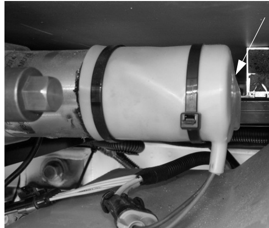
Electric Brake Lever (Located on back side of motor/gear assembly cylinder) -Typical View
