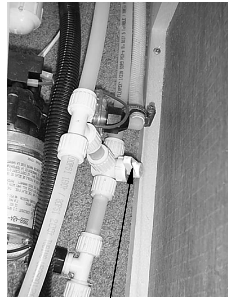
Waterline Drain Valve (Typical)
