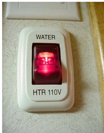
Electric Water Heater Switch (Located near Systems Monitor Panel)
