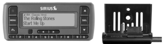
To install the satellite unit, place your Sirius radio into the docking station, aligning the tabs at the edges of the the radio adapter with the grooves in your radio. Gently push the radio down until it is fully seated in the docking station.
