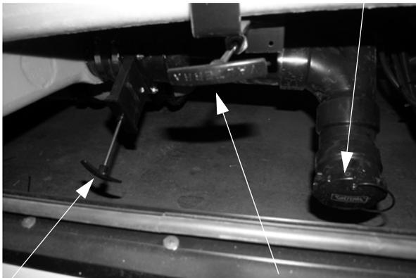
1st - Pull Black Waste Tank Drain valve to drain black water (sewage) tank - then close.
