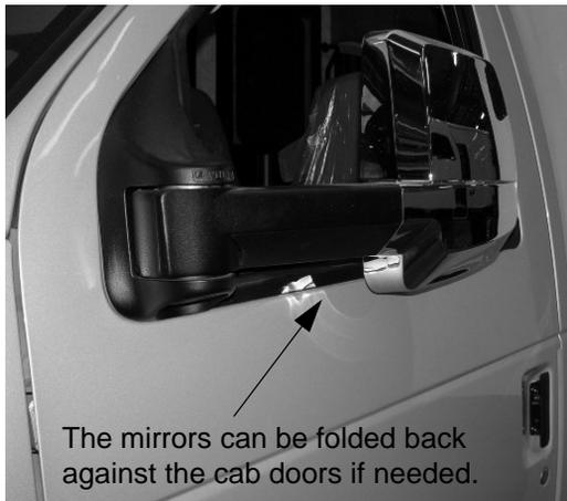
The mirrors can be folded back against the cab doors if needed.
