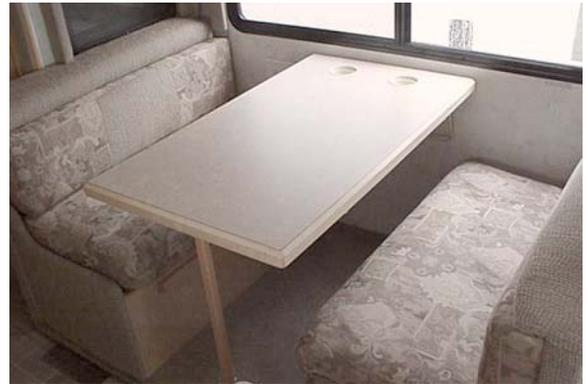
1. Release the catch on the table leg brace and fold the leg up against the bottom of the table.
