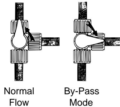
Leave bypass valve handle in NORMAL FLOW position if draining water and blowing out waterlines. Place in BYPASS position ONLY when using antifreeze solution in waterlines.
