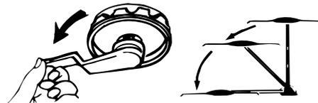
Turn elevating crank (counter-clockwise) in "DOWN" direction until resistance is noted (approximately 13 turns). Antenna is now locked in travel position. Turn amplifier power switch "OFF".
