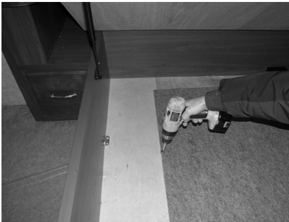
Removable Panel (if equipped) (Located underneath bed) * Lift bed board to access -Typical View
