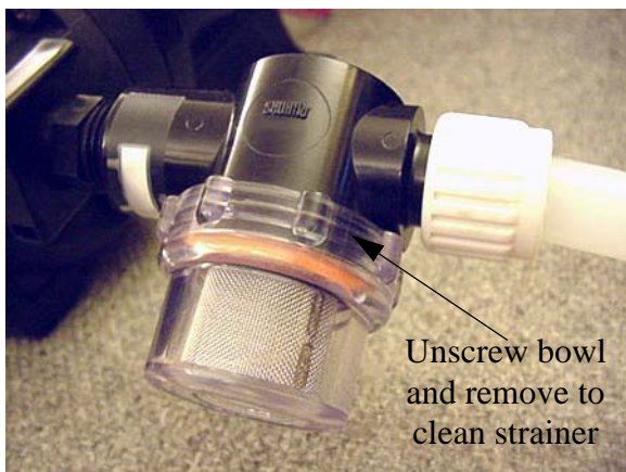
Water Pump Strainer -Typical View
