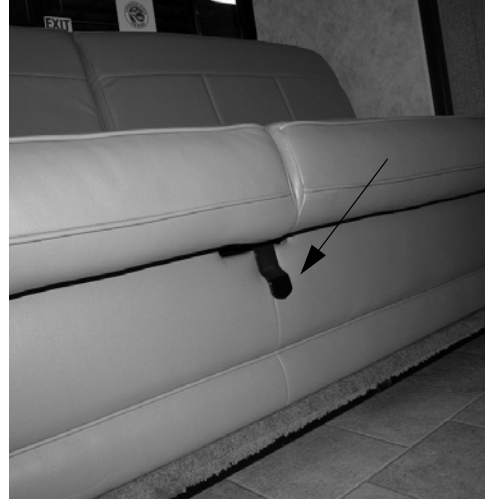
Security Latch (Located on front of sofa) - Pull OUT to release
