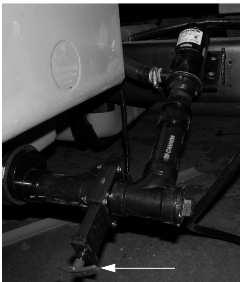
Gray Waste Tank Drain Valve (Located beneath driver side of coach ahead of rear wheel) -Typical View
