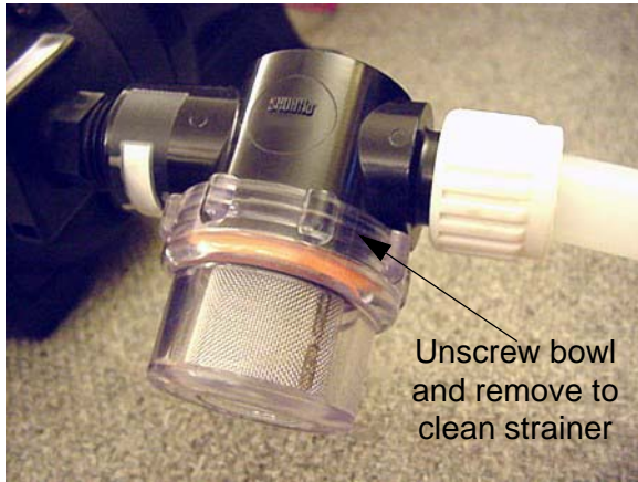
Water Pump Strainer -Typical View
