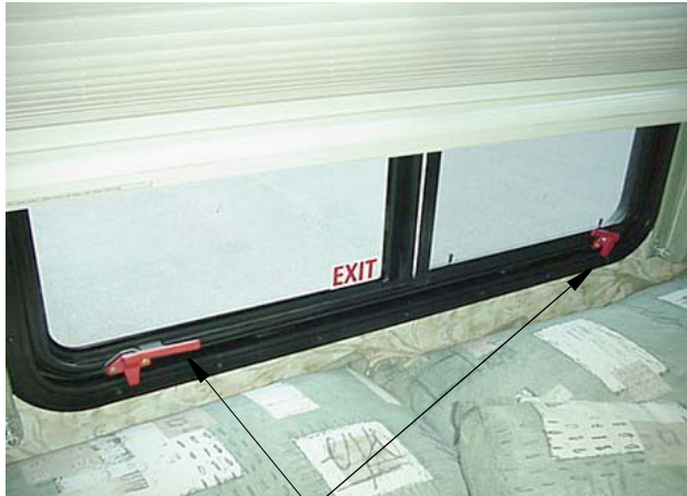
Escape Window - Lift latch handles upward to open
