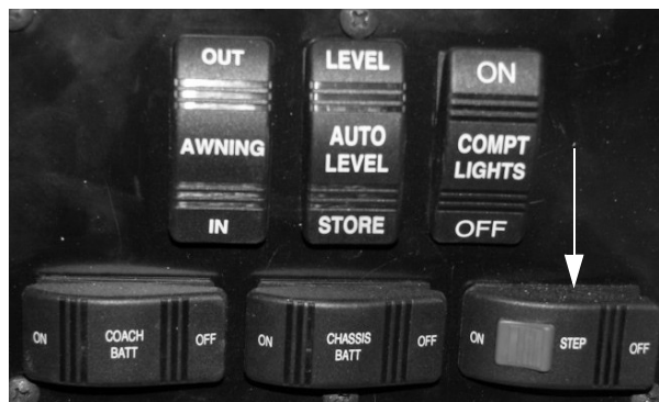
Entry Step Switch (Located near the entrance door) -Typical View
