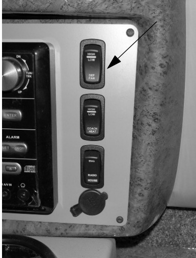
Defrost Fan Switch -Typical View
