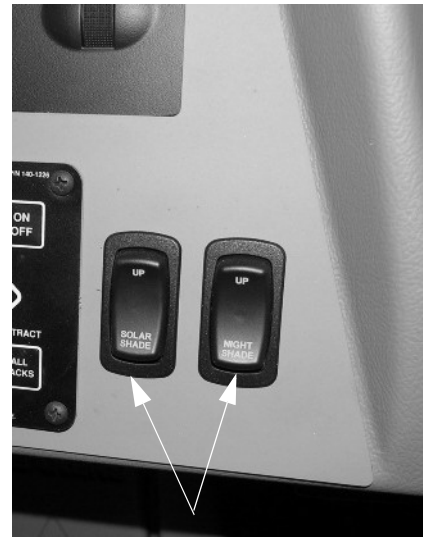
12-Volt Front Drop-Down Solar/ Night Shade Switches (Located on dash) -Typical View
