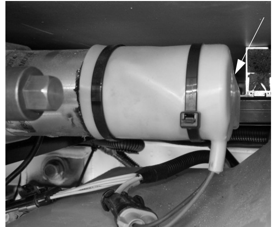
Motor Brake Lever (Located on back side of motor/gear assembly) -Typical View
