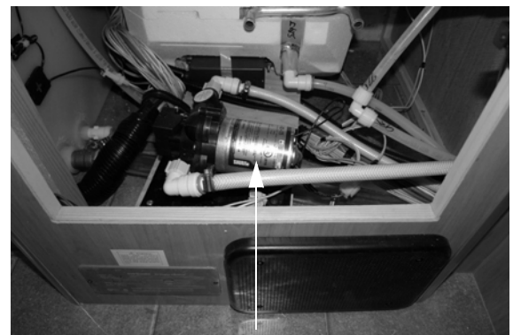
Water Pump (Located behind removable access panel below wardrobe) -Model 24J Shown
