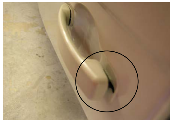
Door Unlatched (note gap)
