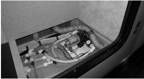
Water Pump (Located beneath removable access panel in passenger rear compartment) -Model 24K Shown
