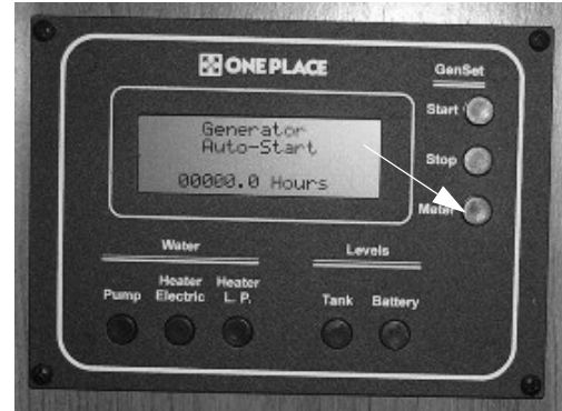
Generator Hourmeter Button -Typical View
