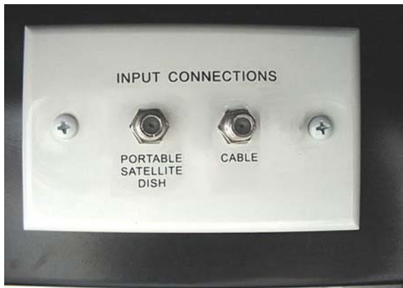
Cable TV and Satellite Connections (Located in shoreline compartment)
