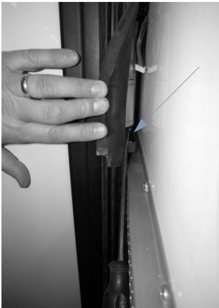
Slideout Motor (Located behind slideout wipe seal)
