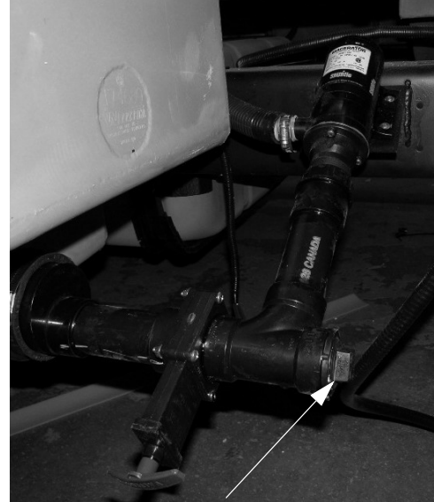
Waste Pump Drain (Located on driver side of coach ahead of rear wheel) * Model 26Q only
