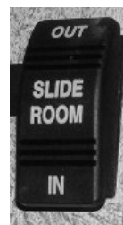
Slideout Switch (Your coach may have one or more slideout switches depending on model, options, and available equipment) -Typical View
