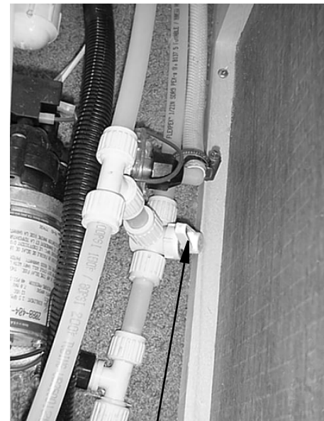
Waterline Drain Valve (Typical)
