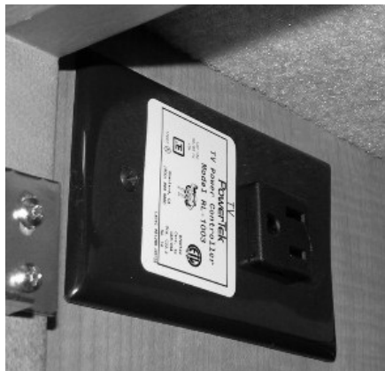
Front TV Ignition Switch Interlock -Typical View
