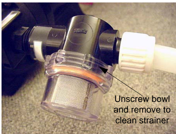
Water Pump Strainer -Typical View
