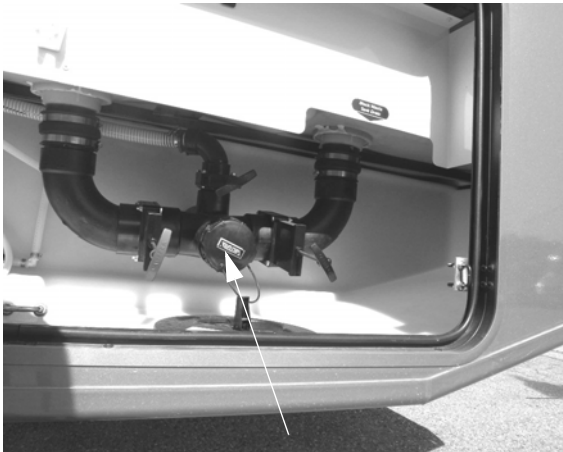
Sewage Drain Outlet (Located in water service center) -Typical View
