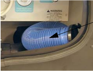
Sewage Drain Hose -Typical View
