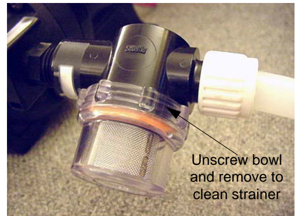
Water Pump Strainer -Typical View
