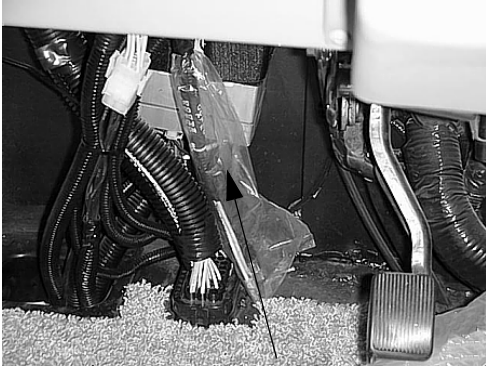
CB Power Wires (in plastic sheath)
