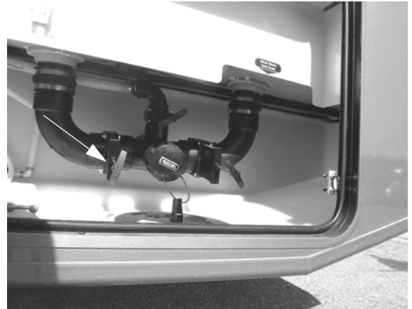
Gray Waste Tank Drain Valve (Located in water service center) -Typical View
