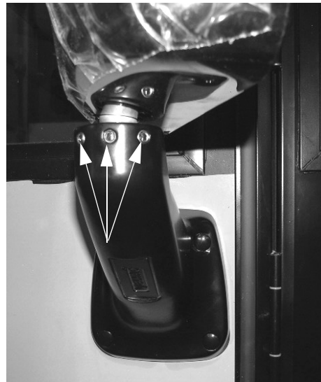
Mirror Head Pivot Lock • Loosen Allen head set screws to pivot mirror head. • Torque 75-100 in./lbs.
