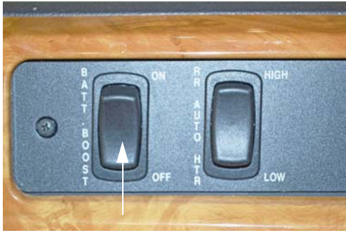
Battery Boost Switch
