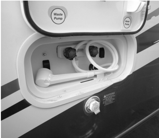
Exterior Shower/Wash Station -Typical View
