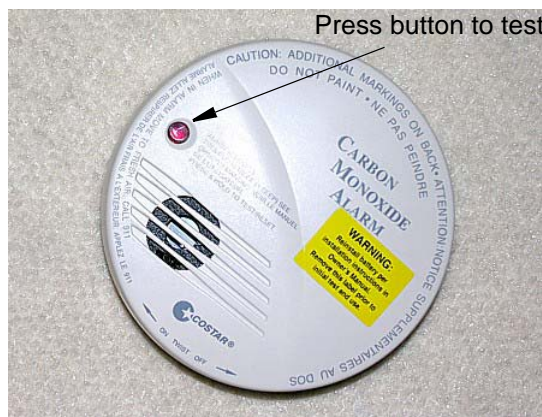
Carbon Monoxide Alarm
