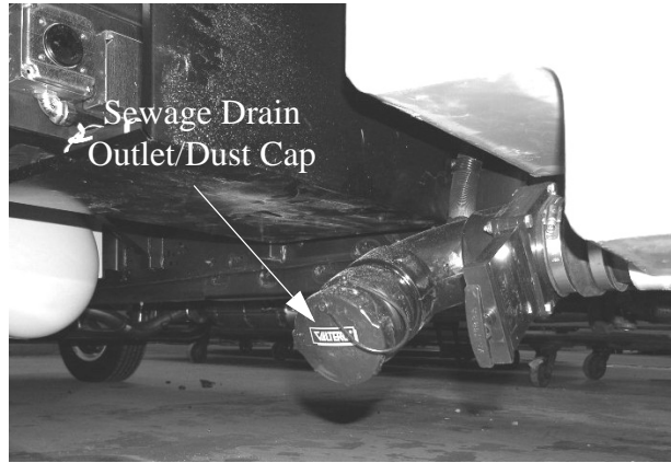
Sewage Drain Outlet/Dust Cap (Located beneath coach on mid-driver side) -Typical View
