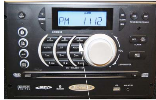
Exterior Speaker Switch "Speaker C" (Located on the interior stereo radio)
