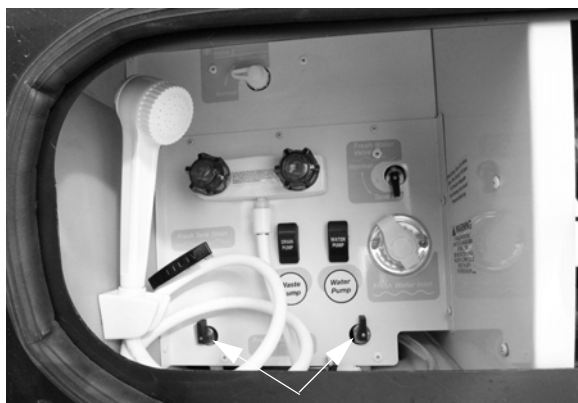
Waterline Drain Valves -Typical View
