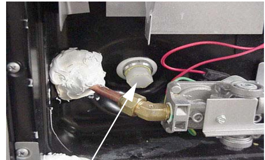
Water Heater Drain Plug (Remove with socket)
