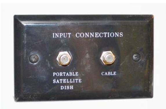
Cable TV and Portable Satellite Connections (Located in the utility or shoreline compartment depending on model.)
