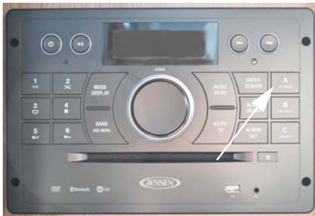
Interior Speaker Switch “SPEAKER A”
