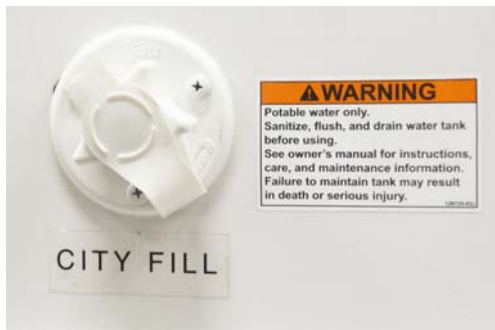
Fresh (City) Water Inlet -Typical View
