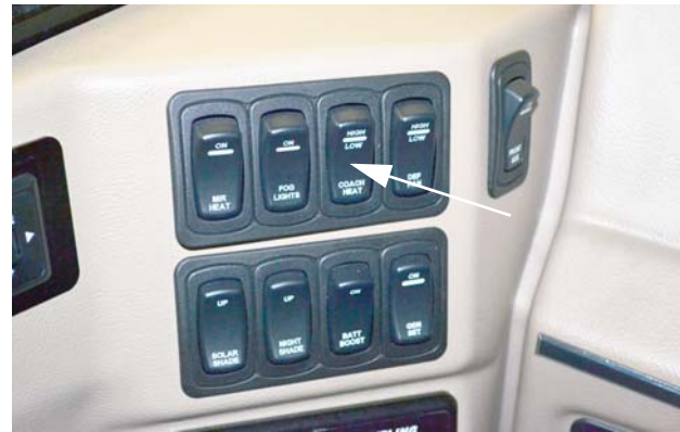
Coach Heat Switch (Located on driver side dash) -Typical View
