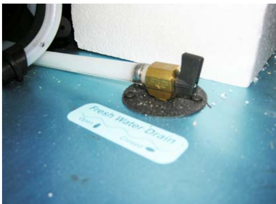
Water Tank Drain Valve - Typical Installation
