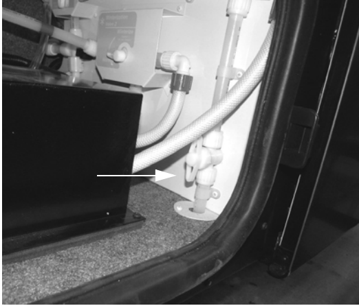
Waterline Drain Valve - Typical Installation
