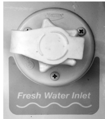
Fresh (City) Water Connection “Fresh Water Inlet” (Located in the water service center)
