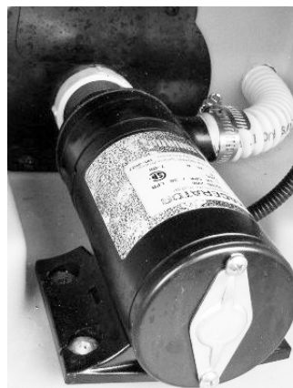
Waste Pump (Located beneath coach) -Typical View
