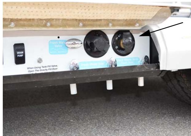
Black Waste Tank Flush Inlet (Located in water center compartment on the driver side of motorhome) -Typical View
