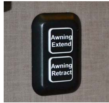
Power Awning Switch (Located near sliding entrance door) -Typical View
