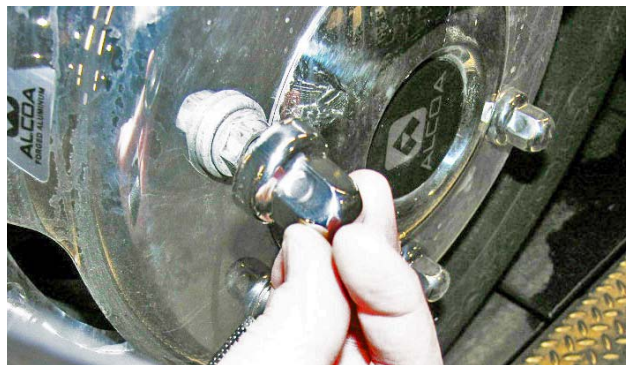
Remove the push on nut covers.
