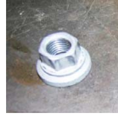
Six Chassis Supplied Lug Nuts with attached washers (located in the co-driver foot well compartment)
