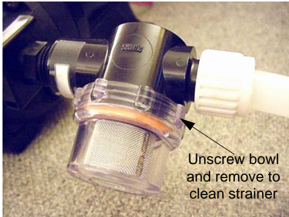
Water Pump Strainer -Typical View
