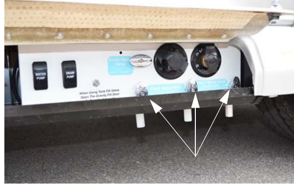
Waterline Drain Valves -Typical installation shown (See the “Water System Drain Valve Locations” chart at the end of this section for locations on your model)
