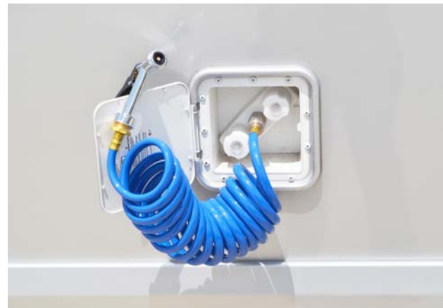
Exterior Shower/Wash Station (Typical)
