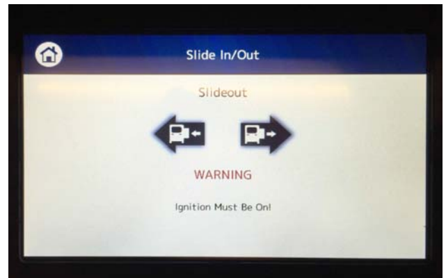
Slideout Switch (Located on Monitor Panel)
