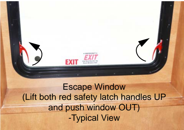
Escape Window (Lift both red safety latch handles UP and push window OUT) -Typical View
