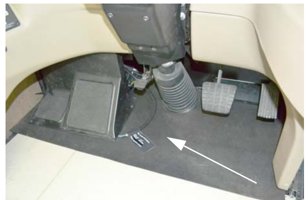
CB Power Wires -Typical View
