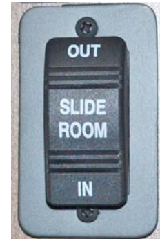
Slideout Switch -Typical View
