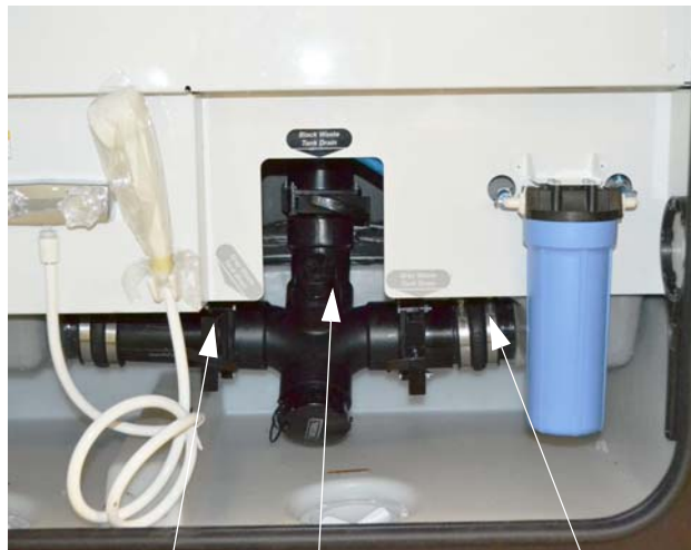
Gray Waste Tank Drain Valve Black Waste Tank Drain Valve Gray Waste Tank Drain Valve
