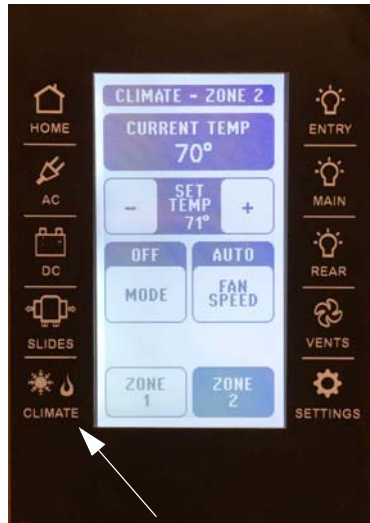
Thermostat “Climate” Screen (Located on Multiplex Monitor Panel)
