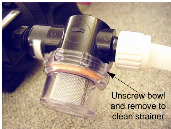
Water Pump Strainer -Typical View
