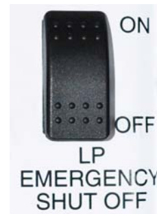
Main Tank Shutoff Switch (Located in driver side compartment) -Typical View
