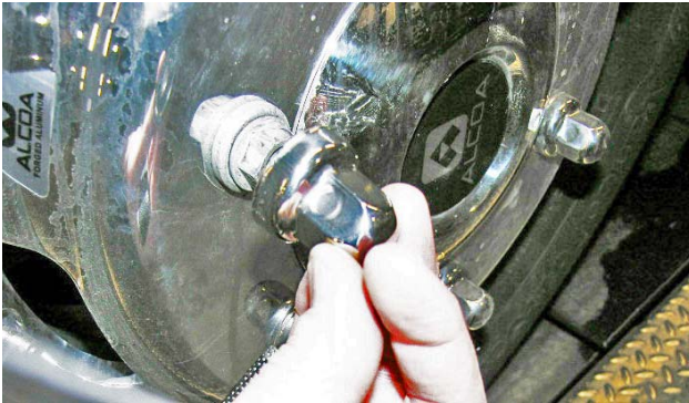
Remove the push on nut covers.
