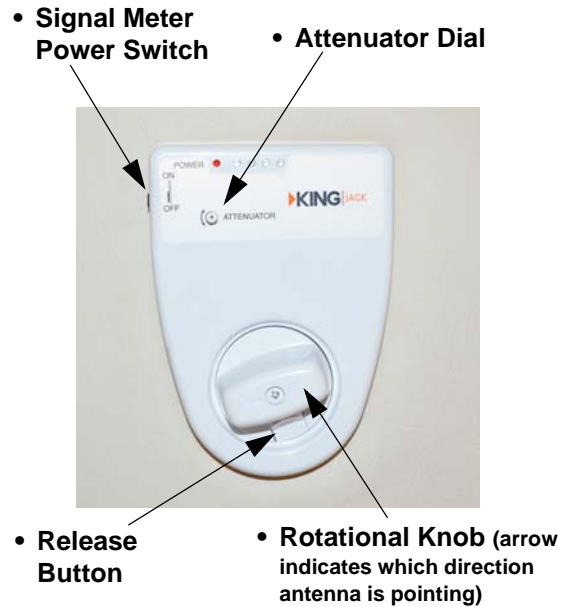
Digital Antenna Signal Meter (Located on ceiling)
