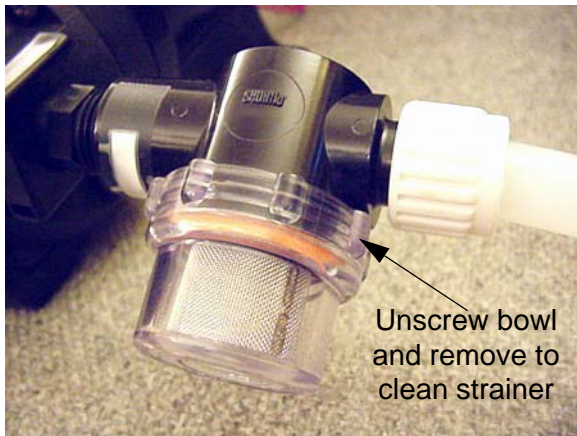
Water Pump Strainer -Typical View
