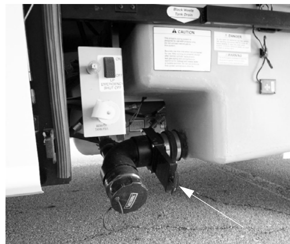
Black Waste Tank Drain Valve (Located in driver side compartment) -Typical View
