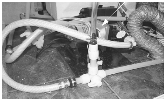
Water Pump (Located beneath driver side rear bed adjustable headrest) -Model 24V shown
