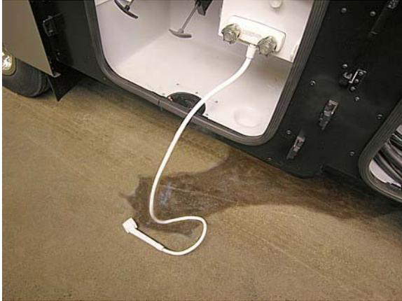
Using exterior shower to drain waterline
