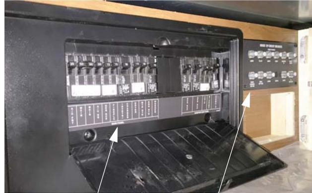
120-Volt House Circuit Breakers      12-Volt House Circuit Breakers
