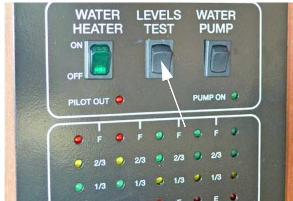
The approximate fluid levels are measured by electronic sensors on the sides of the tanks. There is generally more fluid in a tank than indicated on the monitor panel.
