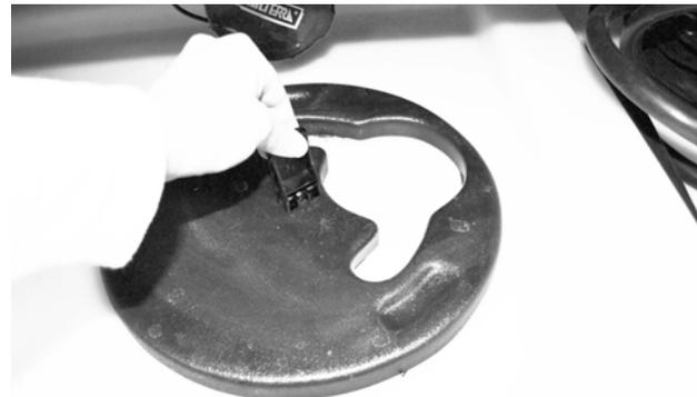
2. Rotate the cover to the largest hole to pass the cord end through.
