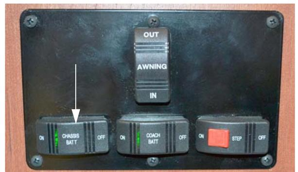
Chassis Battery Disconnect Switch
