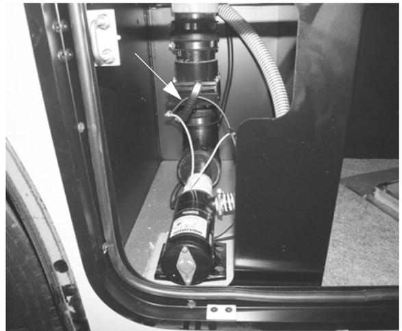
**Black Waste Tank Drain Valve #1 (Front)**
