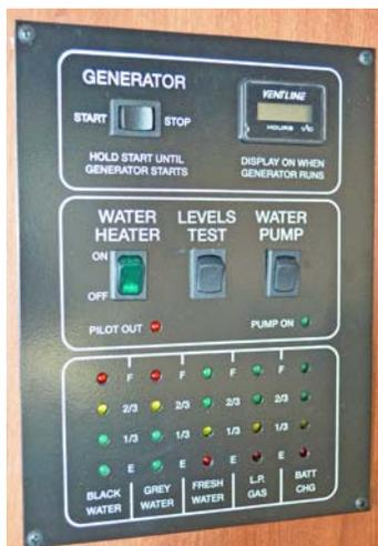
At the touch of a button, this panel will display the fresh water and holding tank levels, propane gas tank level, plus the house battery condition. You can start the generator or turn on the water pump and water heater. Indicator lights tell you if the water pump is on or if the water heater pilot light is out.
