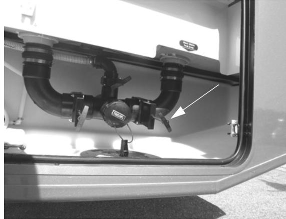
Black Waste Tank Drain Valve (Rear)
