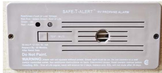
Propane Gas Leak Detector
