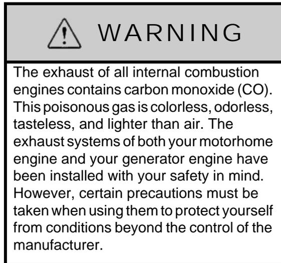
1. Do not simultaneously operate the generator and a power vent, which could draw exhaust gases into the vehicle.
