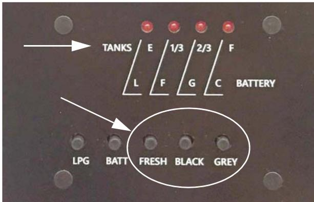
The approximate fluid levels are measured by sensors on the sides of the tanks. There is generally more fluid in a tank than indicated on the monitor panel.
