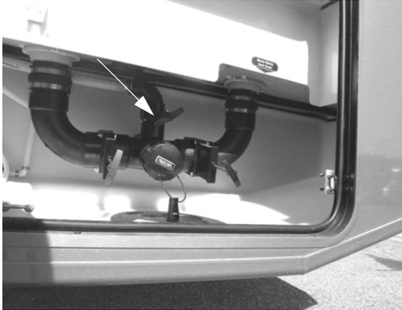
Black Waste Tank Drain Valve #2 (Front)
