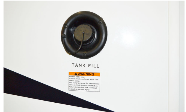
Water Tank Gravity Fill -Typical View
