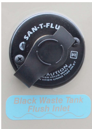
Black Waste Tank Flush Inlet (Located on left sidewall) -Typical View
