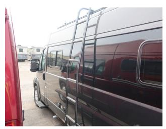
Shown with Ladder properly mounted on rail at driver side.
