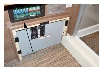
House 12-Volt Fuses (Located on right side twin bed cabinet at rear) -Typical View
