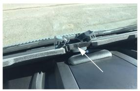
3. Lift each track and lock into place above the windshield.
