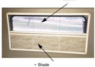
To lower translucent screen, pull the bottom of the screen straight down until the bottom latch "clicks" into position.
