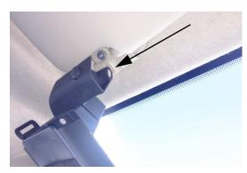
4. Lift the windshield pleated blind at the center handle to raise the shade into the fully extended position. If needed, adjust the rear view mirror to clear the shade.
