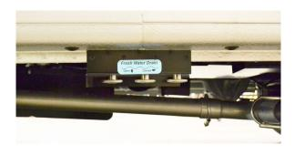
Waterlines and Tank Drain Valves
