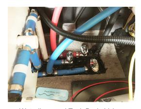
Waterlines and Tank Drain Valves
