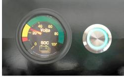
Pure<sup>3</sup> State of Charge (SOC) Gauge (Located on an interior cabinet)
