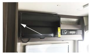
Grasp TV and disengage from wall mounting bracket.
