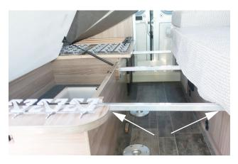
4. Place table top onto the support bars making sure the notch on the bottom of dining table aligns to the support bar.
