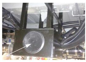
Waste Pump Enclosure (Located beneath motorhome)
