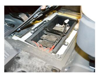
**Chassis Battery Access** (Located beneath driver side floor mat) -Typical View
