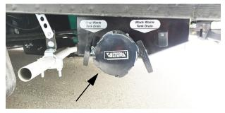
Sewage Drain Outlet (Located beneath motorhome) \*Model 59GL
