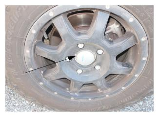
Tire centering ring is clearly visible if it is installed.
