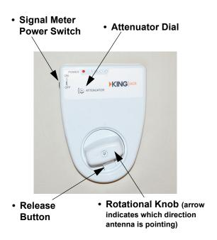
Digital Antenna Signal Meter (Located on ceiling)
