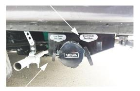
2nd - (Refer to Step 5) Pull Gray Waste Tank Drain valve to drain gray water (sink/shower).
