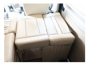
7. Remove support bar from underside of cushion (located above front driver and passenger seat overhead). Attach the support bar (velcro side up) to the notch in side facing dinette seat base and front of galley cabinet.
