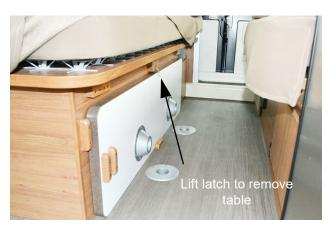
2. Slide the two (2) bed extension support bars (located on the face of the driver side twin bed cabinet) to align with the notch on the passenger side twin bed cabinet.
