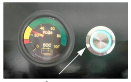
Pure<sup>3</sup> ON/OFF Button (Located on an interior cabinet) -Typical View
