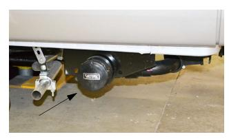
Sewage Drain Outlet (Located beneath motorhome) \*Model 59KL
