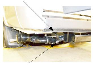
• **2nd** - Pull Gray Waste Tank Drain valve to drain gray water (sink/shower), then close.
