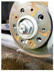
Tire centering ring placed on tire (wide edge toward the hub side).
