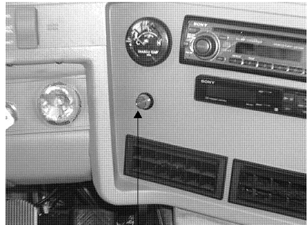
“Check Antenna” Light
