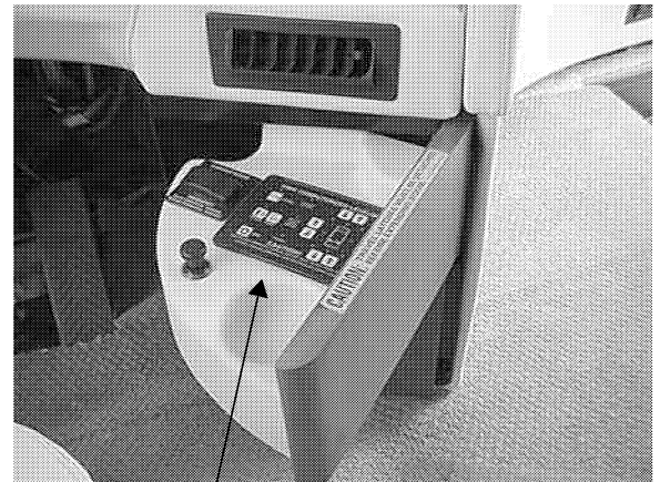
Automatic Leveling System Control Panel
