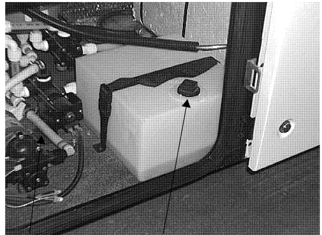
Water Pump RV Water System Antifreeze Reservoir (Remove plug to fill)
