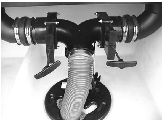
Drainage Hose routed through passage in compartment
