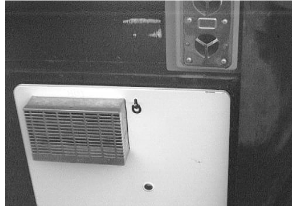
Water Heater Service Access Panel
