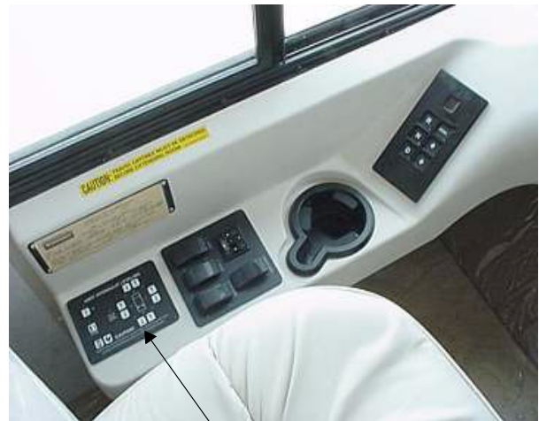
Leveling System Control Panel
