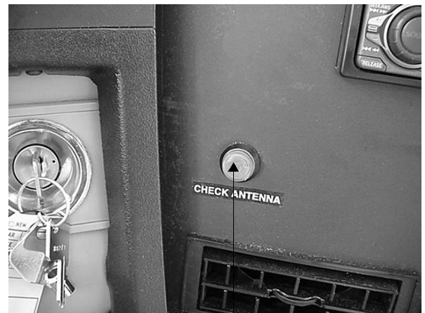
“Check Antenna” Light
