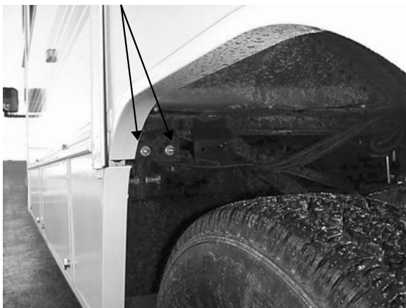
Rear Air Spring Valves located inside left rear wheelwell
