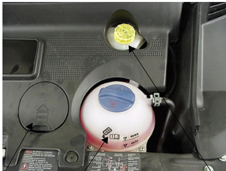
Oil Fill Access
