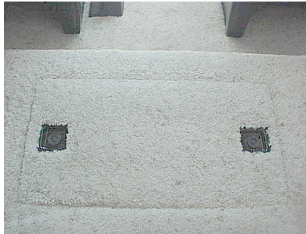
House Battery Storage (in floor behind front seats)
