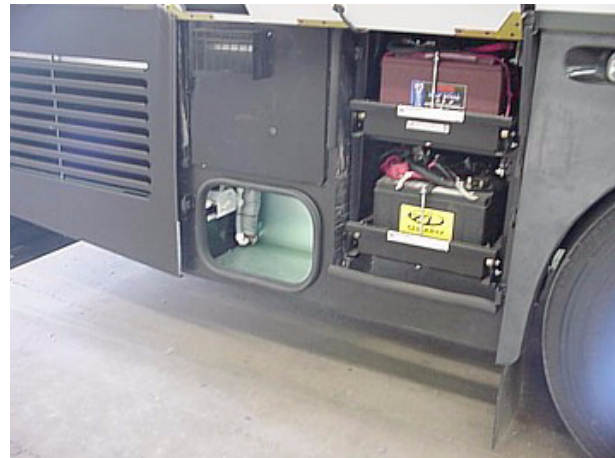
Water Heater Service Access Panel
