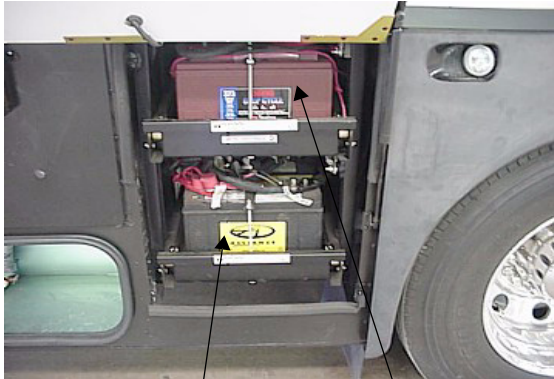
Chassis Batteries House Batteries
