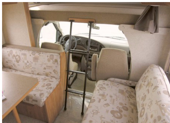
Front Overhead Bunk Shown with bunk sections and ladder in use position
