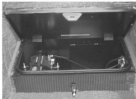
House Battery Storage in Entrance Step
