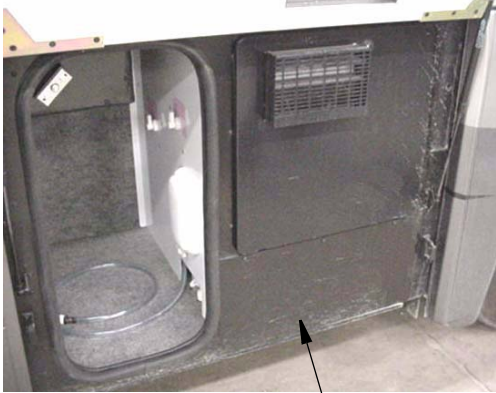
Water Pump Access Panel (typical)
