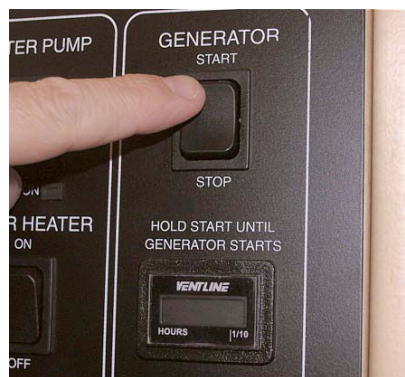
Generator Switch and Hourmeter
