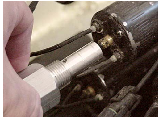
Use 1/4" nut driver built into end of pump reservoir cap to open slideout solenoid valves.
