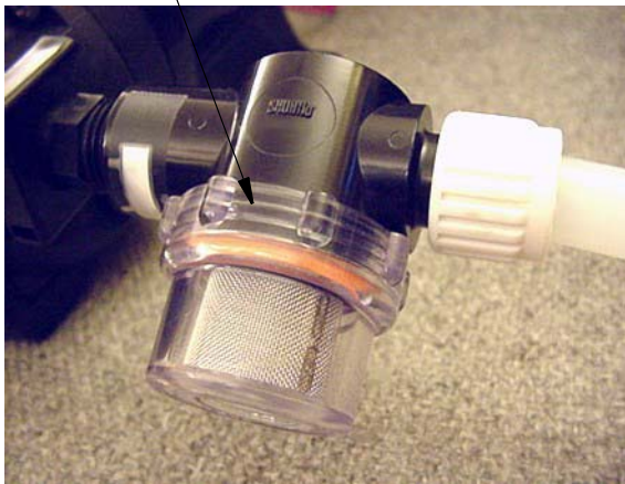
Water Pump Strainer in Water Service Center (typical)
