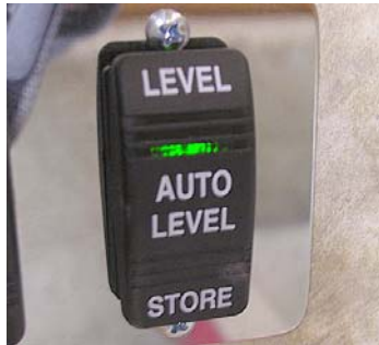
Auto Level Switch inside Entrance Door
