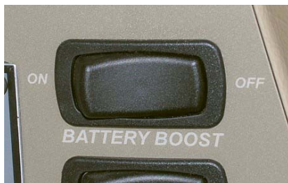
Battery Boost Switch
