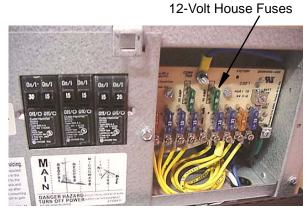
The fuse panel accepts only blade type plug-in fuses. Always replace fuses with those of the same amperage rating.
