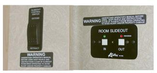
Slideout Switches (typical)
