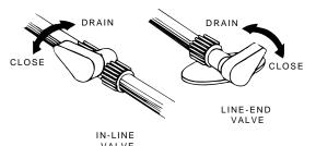
Water Line Drain Valves (Typical)
