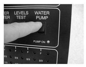
(Some models may also have a pump switch in the water system compartment on the outside of the coach.)
