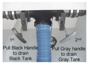
Holding Tank Dump Valves (Typical)
