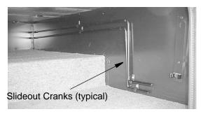
The crank sockets are located behind covers on the lower ends of the room on the outside of the coach. Your coach may have one of the two types of covers shown.
