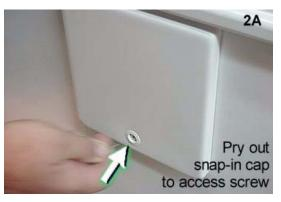
Type B-Single Arm - Cover mounted beneath face of slideout room:
