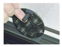
If the window will not open after three or more full turns of the knob, the glass may be stuck to the sealing gasket. Go to the outside of the coach and gently free the glass with your fingers. A periodic light dusting of talcum powder on the gasket should prevent this from recurring.
