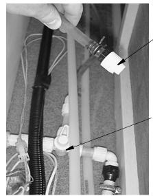
Siphon Tube (insert into container of RV water system antifreeze)
