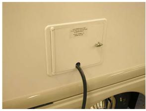
Route power cord through passage and close door while shoreline is connected to outlet.
