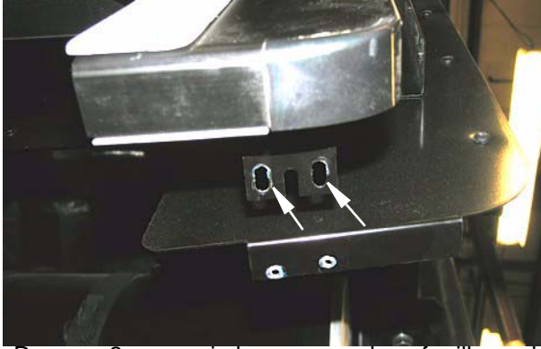
Remove 2 screws in lower rear edge of grill panel shown, then swing hinged panel upward
