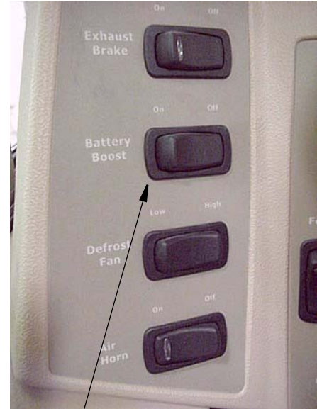
Battery Boost Switch
