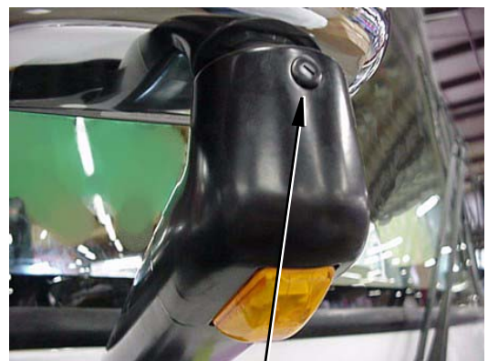
Unscrew protective cap and loosen Allen head set screw to pivot mirror head.
