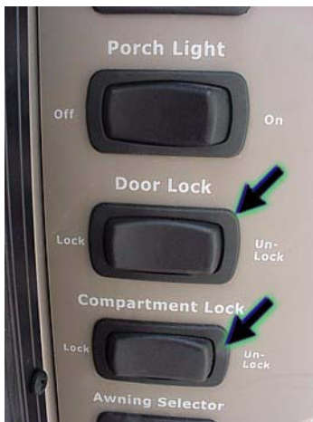
Power Door Locks on entry switch panel
