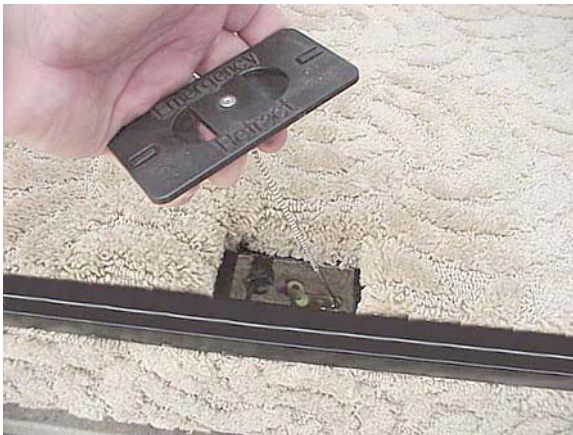
Pull chain to release step mechanism and manually slide step cover back.
