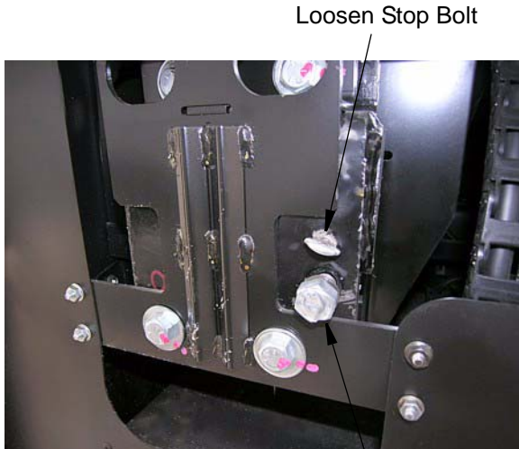
Turn Retract Bolt to crank room in
