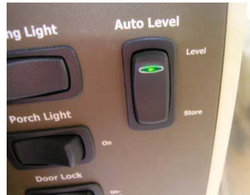
Auto Level Switch inside Entrance Door
