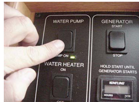
Water Pump Switch on OnePlace Panel
