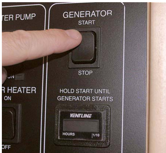
Generator Switch and Hourmeter on monitor panel
