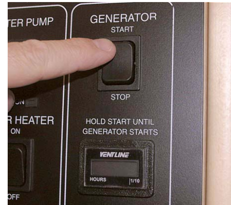
Generator Switch and Hourmeter on Monitor Panel
