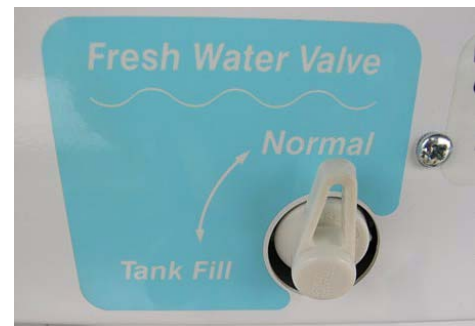
Fresh Water Valve in Normal use position (Located in water service center)
