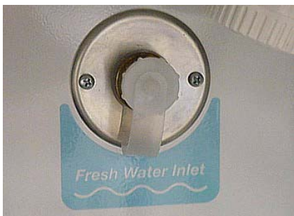
Fresh (City) Water Connection
