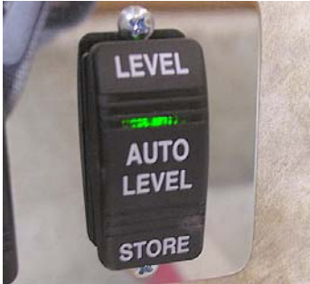
Auto Level Switch (Located inside entrance door)
