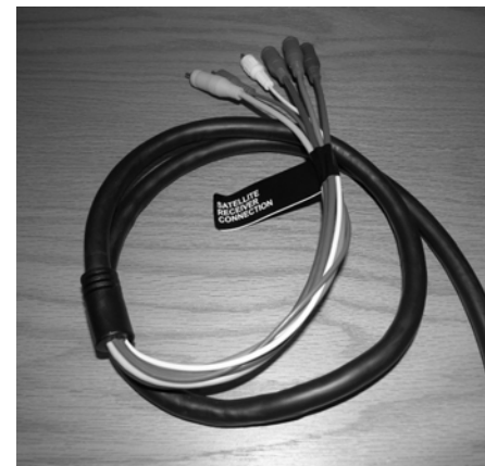
High Definition Accessory Connection Cables (Located in cabinet near TV)
